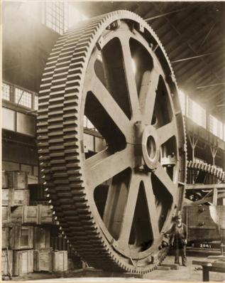
Molded staggered tooth gear
